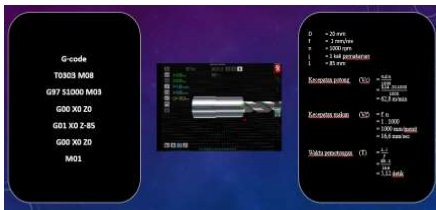
Gambar 5. Proses Drill Diameter 20mm
